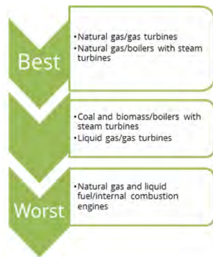
Indicative Relative NO x Emissions Performance of Common CHP Prime mover Technology/Fuel Combinations
